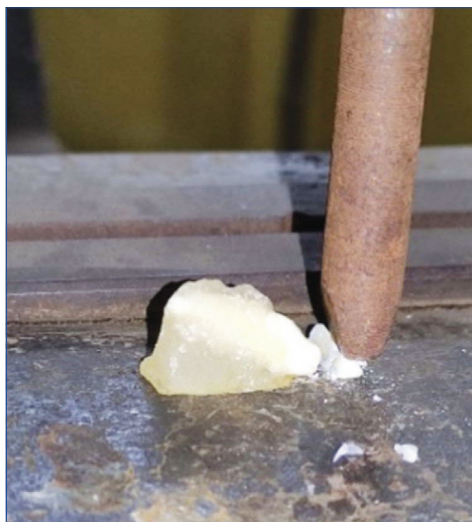
[Table/Fig-4]: Separation of reattached fragment from tooth.
