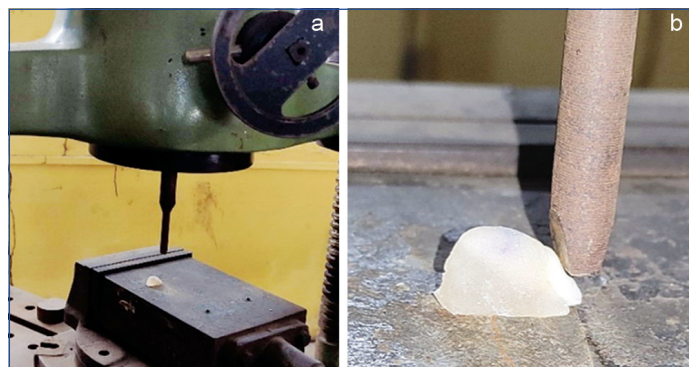
[Table/Fig-3]: a) Specimen embedded in acrylic block were mounted in UTM; b) Rod of the UTM held perpendicular to the long axis of the tooth and also to the palatal surface of the tooth, at the incisal third of the crown.
